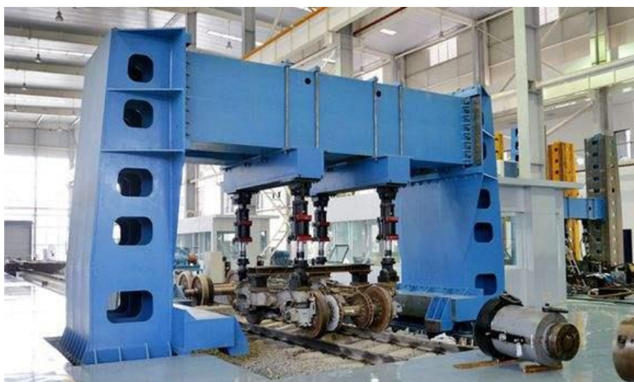
Full-scale multi-functional test platform for track-track system
